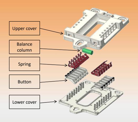
GTUWP-5.0 Panel Connector is mainly assembled by Upper cover, Balance column, Spring, Button, and Lower cover.
